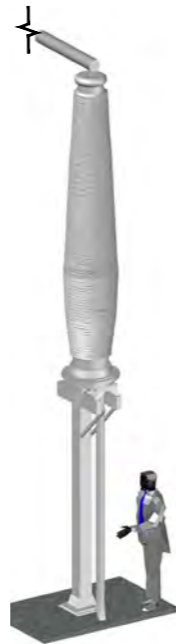
TYPICAL SINGLE CABLE SEALING END
