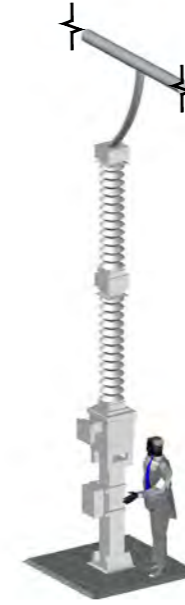
TYPICAL SINGLE VOLTAGE TRANSFORMER
